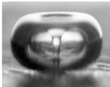
Cavitation bubble ( \mu\text{m} size range)
